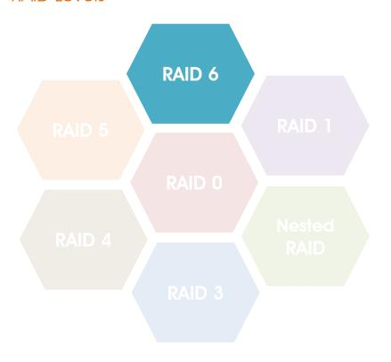
Striped set with independent disk access and dual distributed parity
