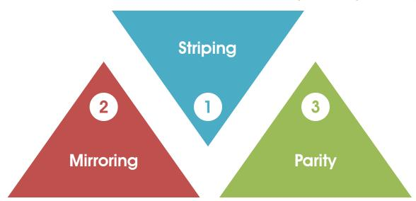
Mirroring is a technique whereby the same data is stored on two different disk drives, yielding two copies of the data.
